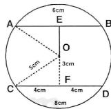
In right triangle COF, by Pythagoras theorem  $(m\overline{OC})^2 = (m\overline{CF})^2 + (m\overline{OF})^2$  $(5cm)^2 = (4cm)^2 + (mOF)^2$  $25cm^{2}-16cm^{2}+\left(m\overline{OF}\right)^{2}$  $9cm^2 = \left(m\overline{OF}\right)^2$
